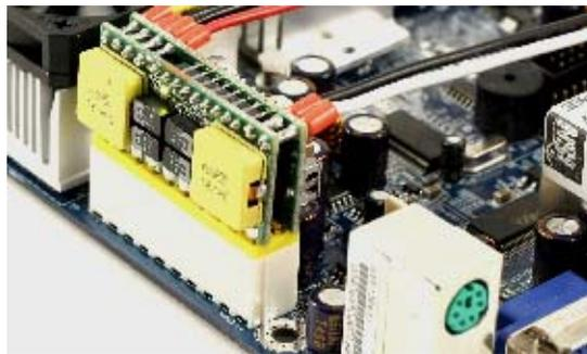
2) Connect a 12 VDC power adapter (or any regulated 12V source) to the DC-to-DC connector, center pin / white wire is positive (+).
